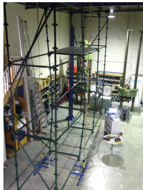
FIG.2 SCAFFOLD UNDER PEAK TEST LOAD
